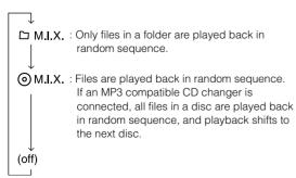
If a CD changer or an MP3 compatible CD changer is connected: After pressing FUNC./SETUP to select the function mode (RPT/M.I.X.), perform the operation within 10 seconds.
